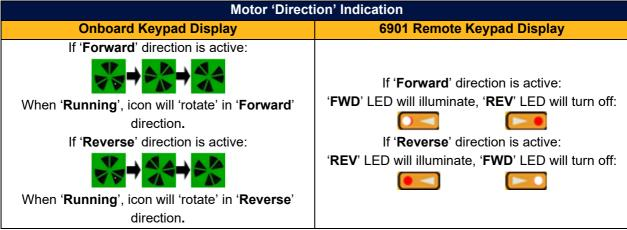
Note: The direction can be changed on the Remote keypad at any time (i.e., when drive is 'Running' or is 'Stopped'.
