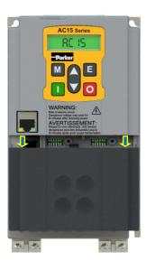
2. Now slide the cover down and pull away from the control module.
