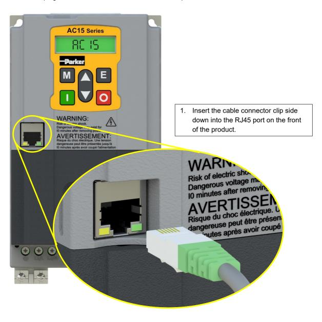
To remove the cable, push the connector clip up towards the cable and pull away from the product.
